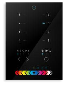
This trully simple controller features an on/off button at the top, 8 buttons to choose from up to 200 lighting scenes (25x8), 2 buttons to cycle between pages and a horizontal fader to instantly adjust dimmer, speed
