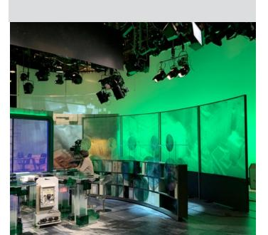
Asymmetric Asymmetric cyclorama powered by LED source in RGBW. Thanks to its sophisticated specifically designed optical system, it allows to illuminate in an absolutely even way an area of over 40 sqm when positioned at a distance from the backdrop of only 1,5m.
